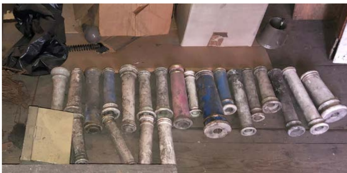
Figures 10: A collection of late-19 th century ceramic and gilt columns found within the building, which would have formed the central part of G. Williamson & Co's beam scales.
