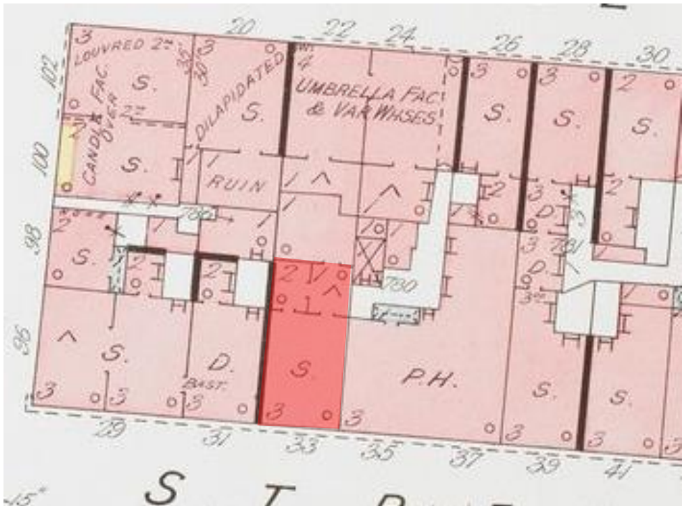
Figure 16: 1888 Goad's Fire Insurance Plan – This detailed plan shows an indicative internal planform arrangement for No. 33, and shows the original 18 th century two-storey outrigger to the rear left of the ground floor (accessed through an internal doorway) and a single-storey extension over the former yard, which shows an internal link into the a larger, single-storey outbuilding in the current location of the open rear yard of the property. The building is marked "S" for "Shop".
