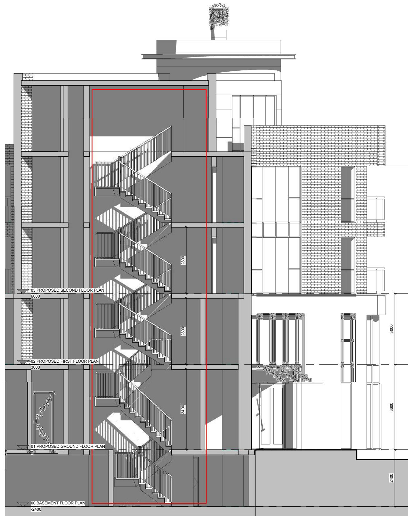
SECTION SHOWING SOUTH STAIRCASE (RESIDENTIAL MAIN ENTRANCE)
