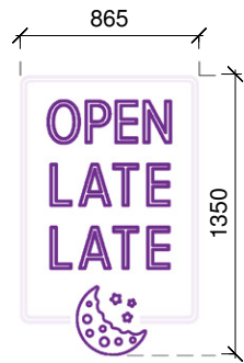
Proposed LED illuminated sign - 3 Location: Located behind shop front glazing, left of entrance Type: Self illuminated LED sign Detail note: Illuminated signage behind glass shop front. Letters to be fixed to horizontal rods behind. Vertical and horizontal aluminium rods 15mm diameter support from existing structure above.
