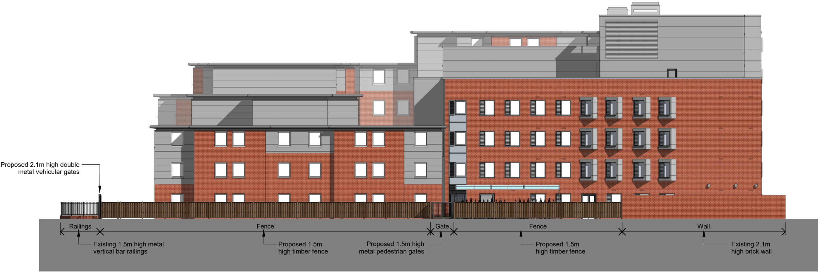
A North East Elevation - Boundary Treatment 1 : 200
