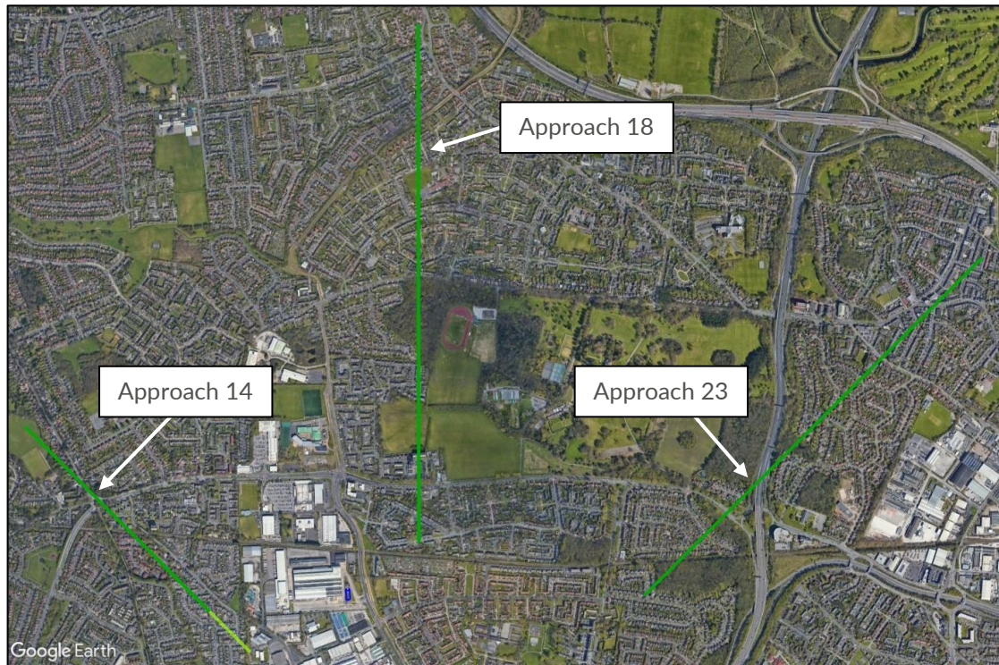
Figure 7 Glare intensities where solar reflections are geometrically possible
