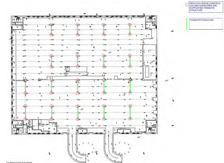
Figure 7.2: Transfer Beams supporting roof trusses
