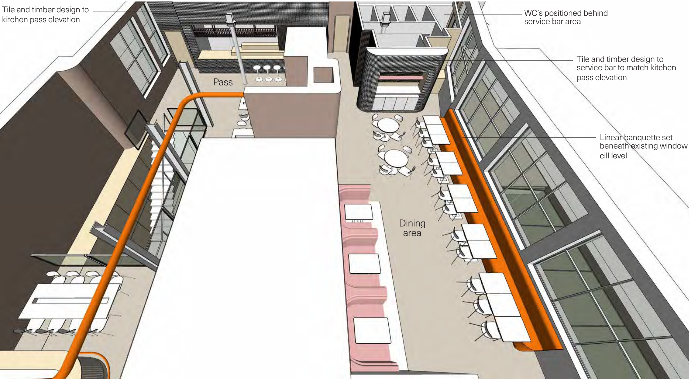
Excerpt from Section GG - showing kitchen pass and service bar frontage facing main dining room
