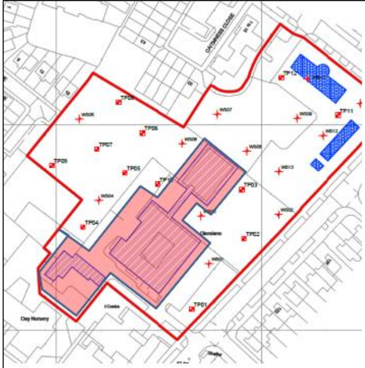
Figure 2: Areas to use concrete class DS-1, AC-1 (white shaded) and DS-2 AC-2 (red shaded)
