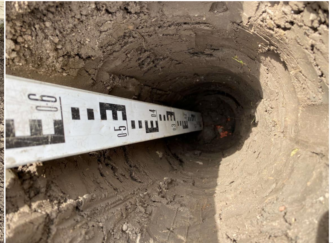
Photographs 5 and 6: Hand Dug Pit Topsoil Depth Validation – HDP17, Plot 28
