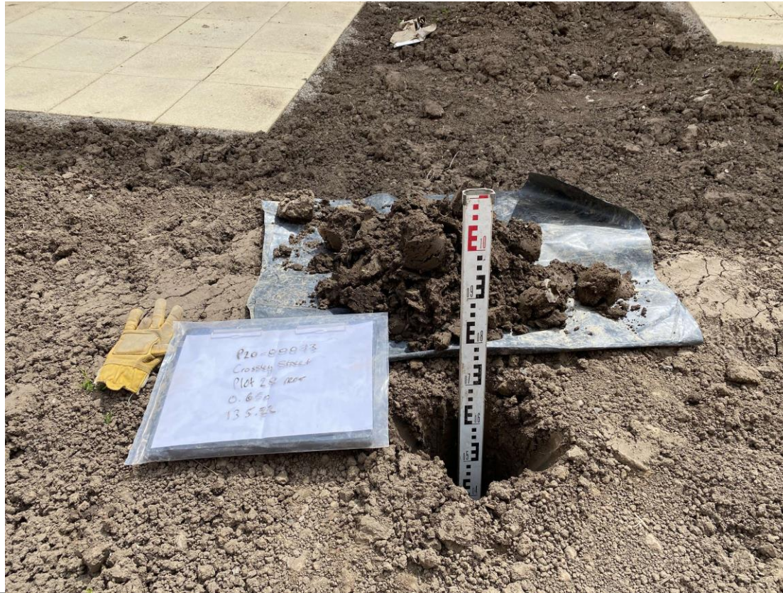
Photographs 5 and 6: Hand Dug Pit Topsoil Depth Validation – HDP17, Plot 28
