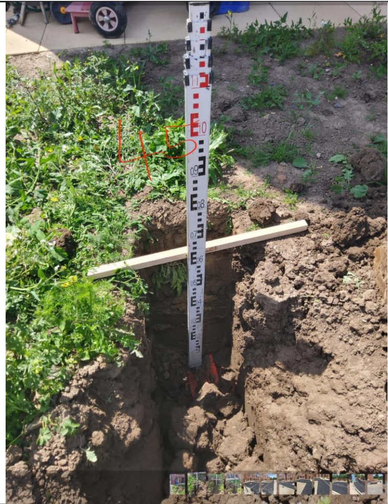
Photograph 22: Trial pit showing 600mm capping overlying high-visibility membrane in front garden area of plot 45.
