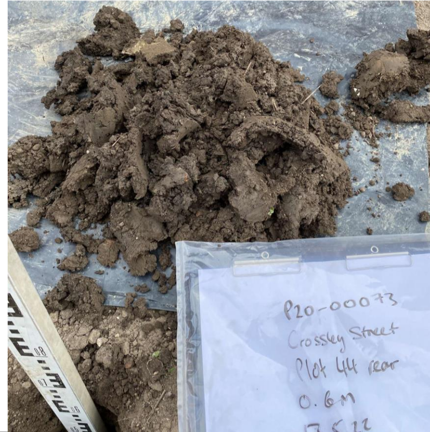
Photograph 1: Hand Dug Pit Topsoil Depth Validation – HDP15, Plot 44
