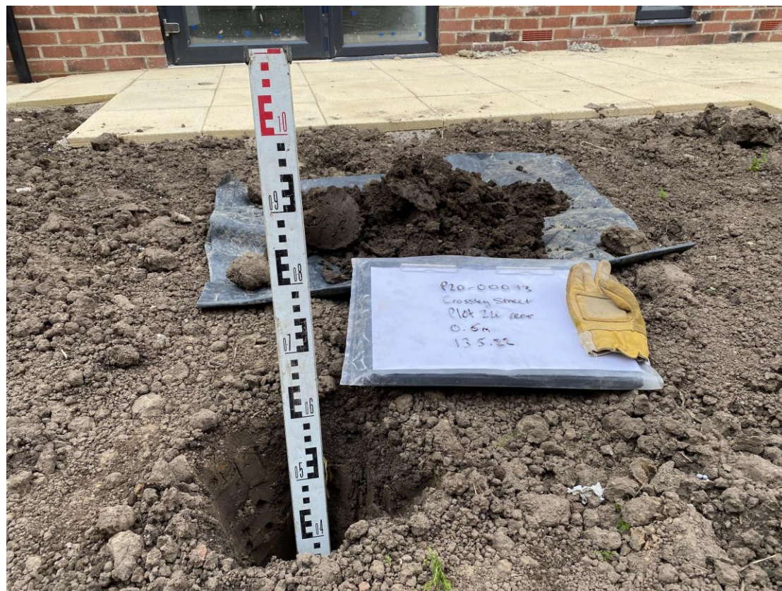
Photographs 7 and 8: Hand Dug Pit Topsoil Depth Validation – HDP18, Plot 24 Rear
