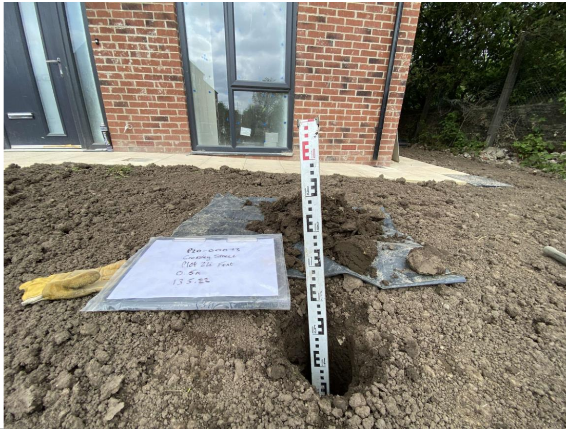
Photographs 9 and 10: Hand Dug Pit Topsoil Depth Validation – HDP19, Plot 24 Front
