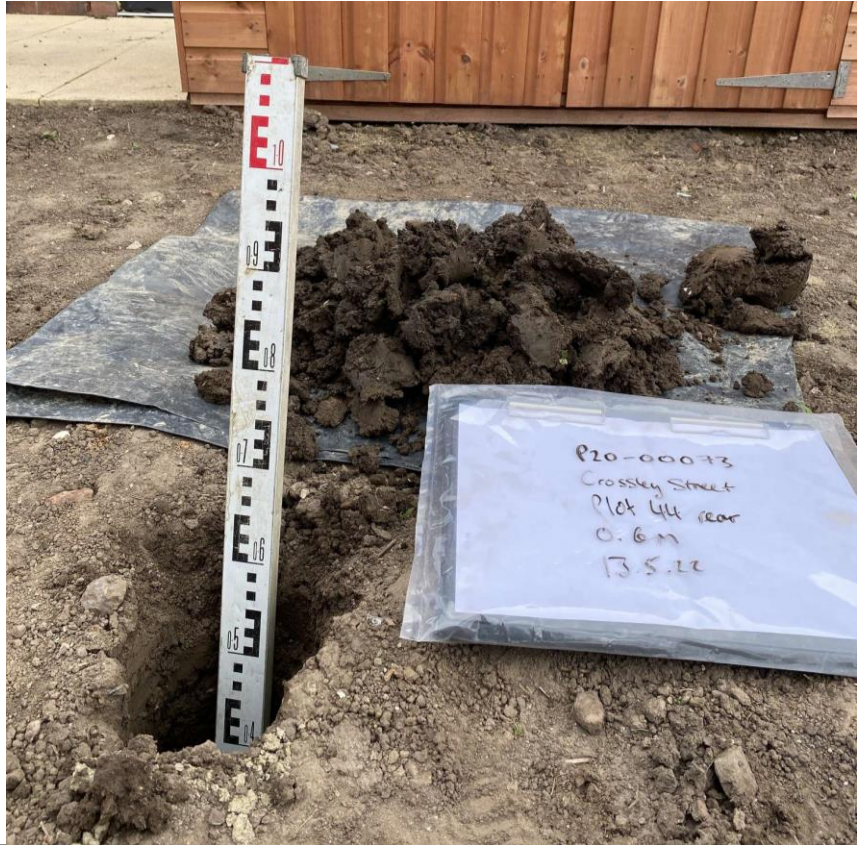
Photograph 1: Hand Dug Pit Topsoil Depth Validation – HDP15, Plot 44
