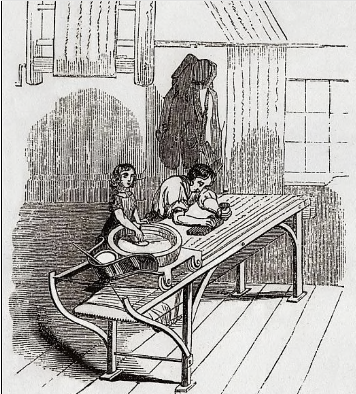
Plate x: Block-printing a design onto a length of calico cloth
