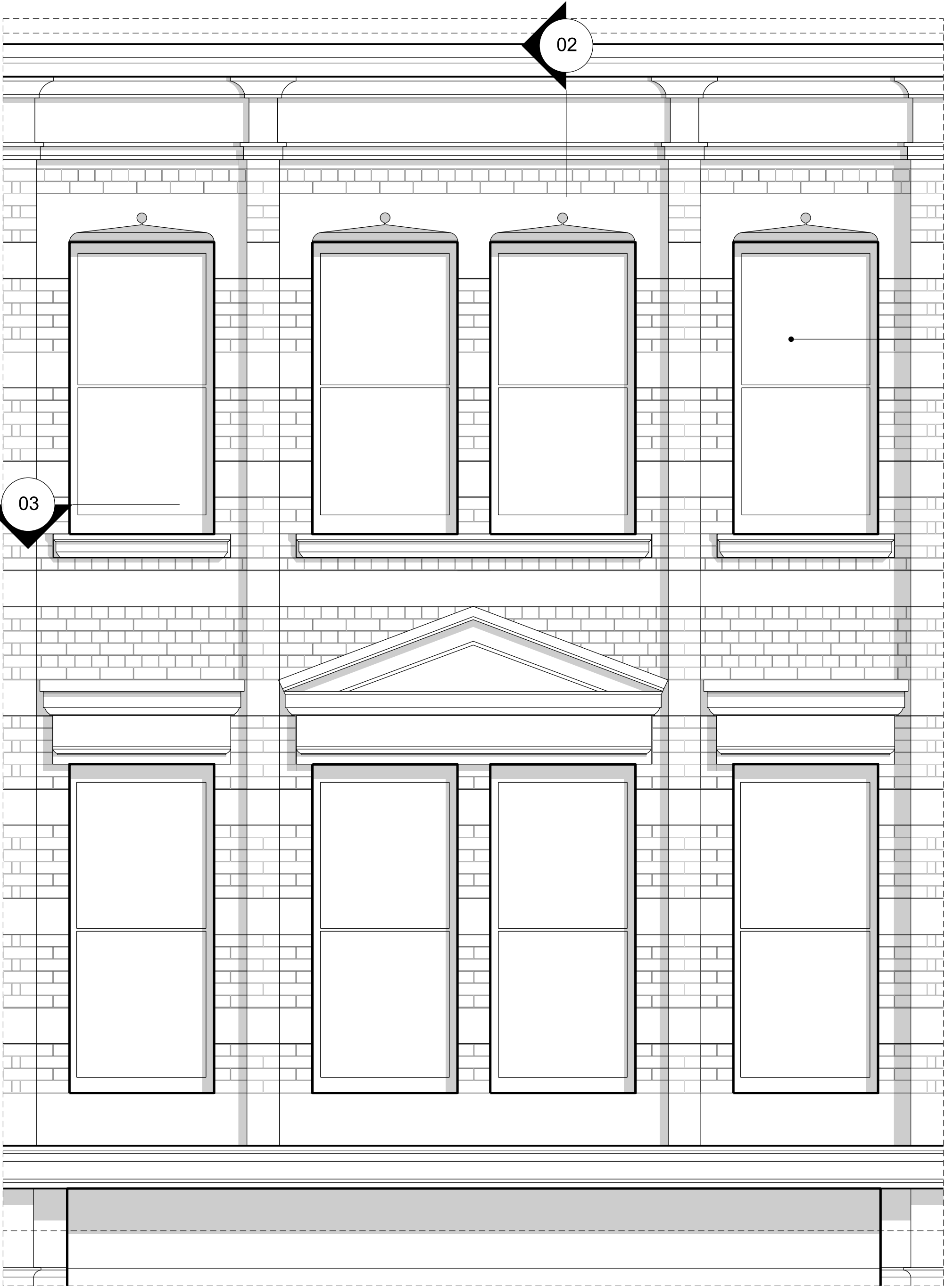
01 Deansgate Timber Sash Window- EXISTING ELEVATION 1:25
