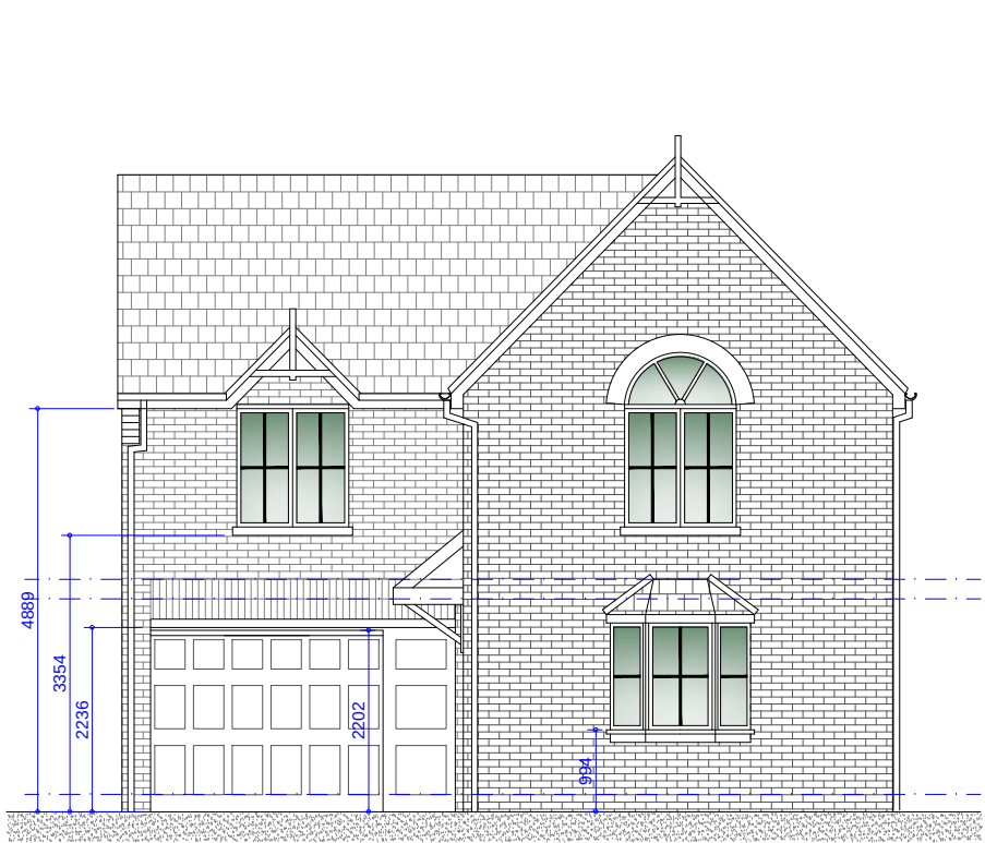
Existing Front Elevation Scale 1:100
