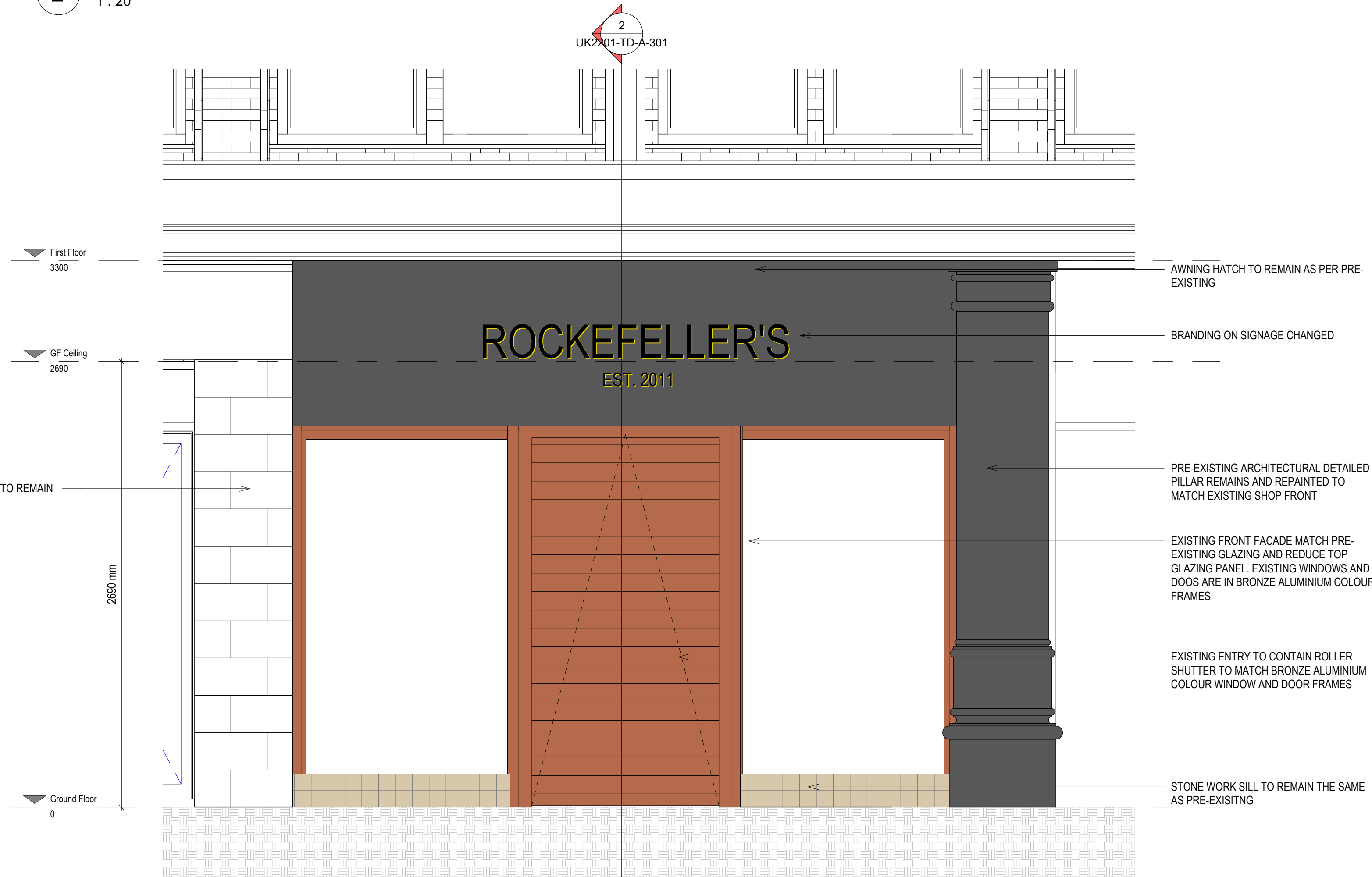
3. EXISTING SHOPFRONT ELEVATION A - CLOSED ROLLER DOOR 1 : 20
