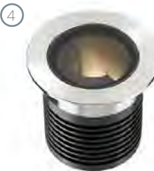
Ground recessed LED uplight. 2700K CCT, min CRI90 500lm; 7W, dimmable Supplied with glare reducing and beam shaping accessories
