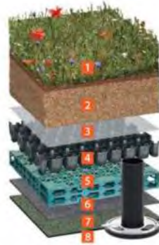
Typical build up of green/blue roof system
