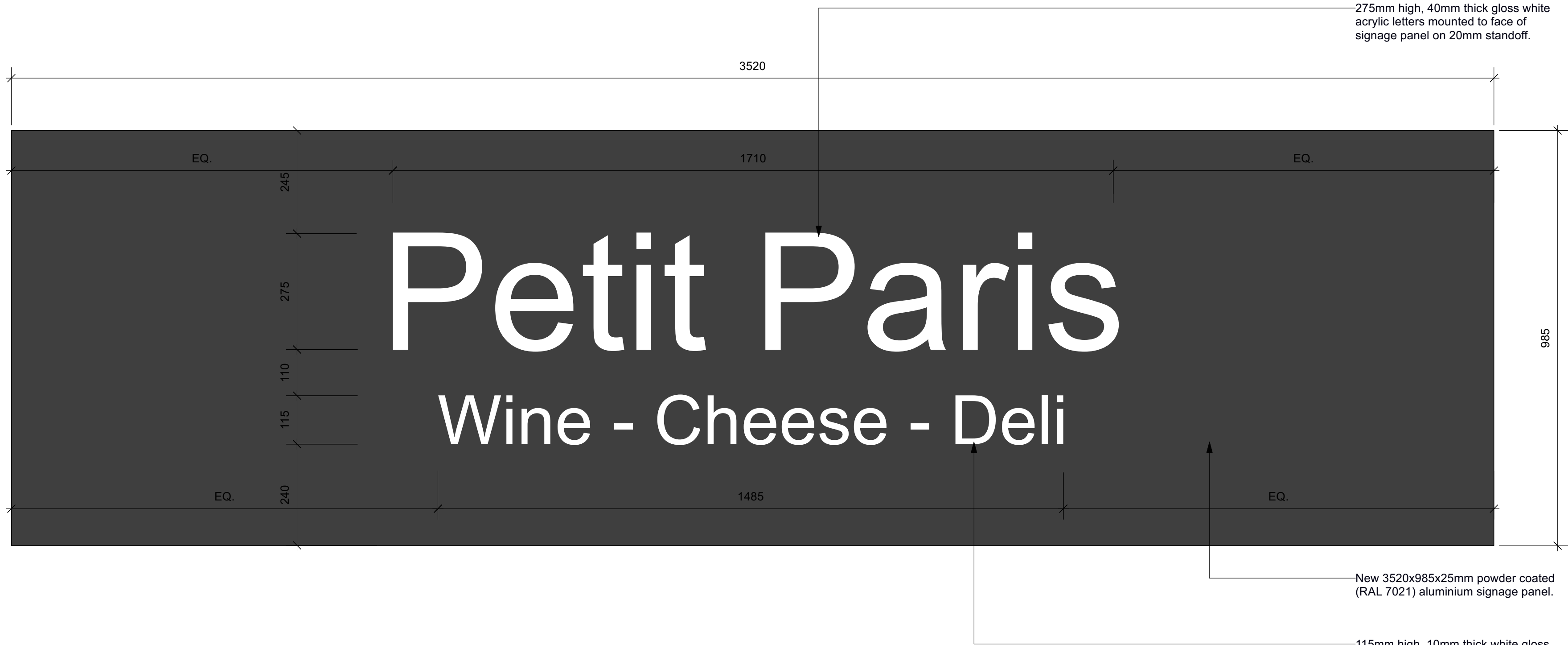
1 SIGNAGE PANEL ELEVATION PL500 SCALE: 1:8@A1
