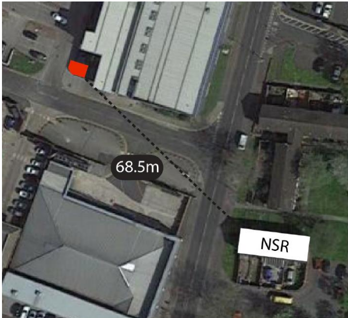
Figure 1: Location of installed plant highlighted in red and closest NSR properties highlighted in white
