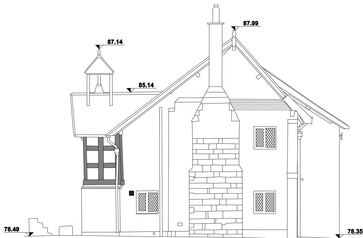
SOUTH ELEVATION AS EXISTING
