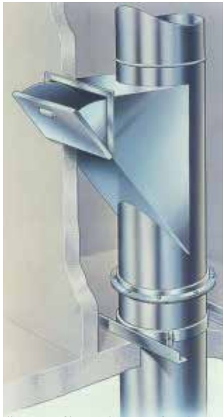
Illustration of hopper door into refuse chute
