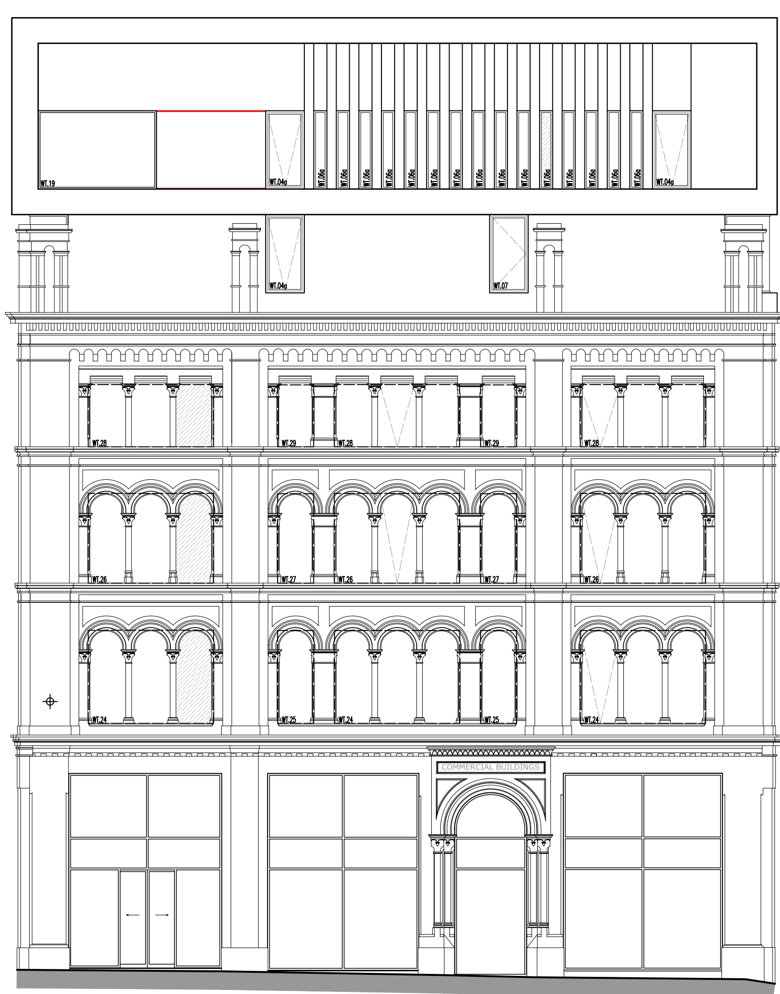
New Glazing at Ground Floor
