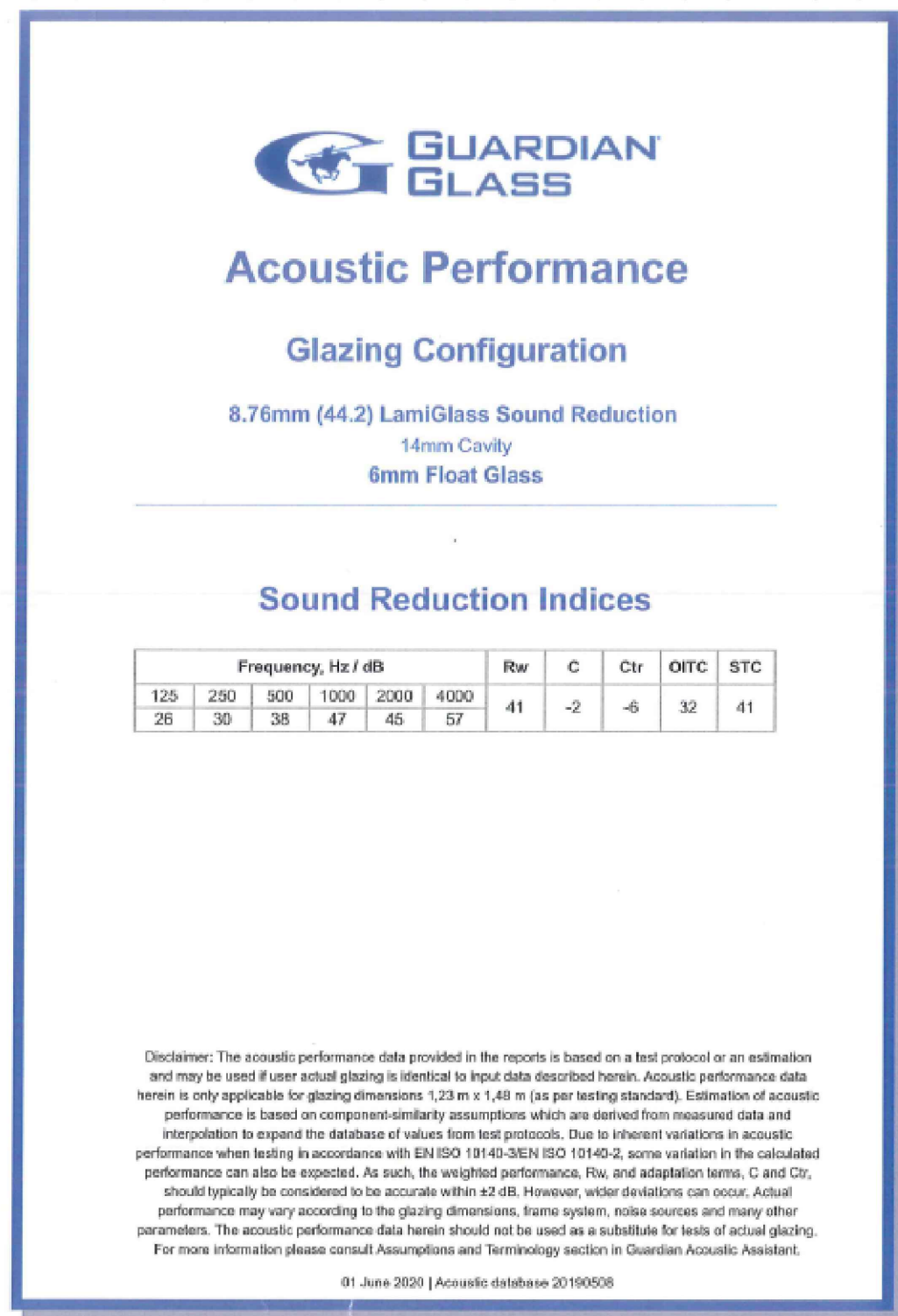
Window manufacturers specification sheet
