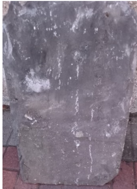
Samples of reclaimed Welsh ton slates for replacement of existing damaged slates (if any)
