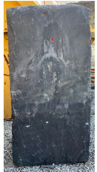
Samples of reclaimed Welsh ton slates for replacement of existing damaged slates (if any)
