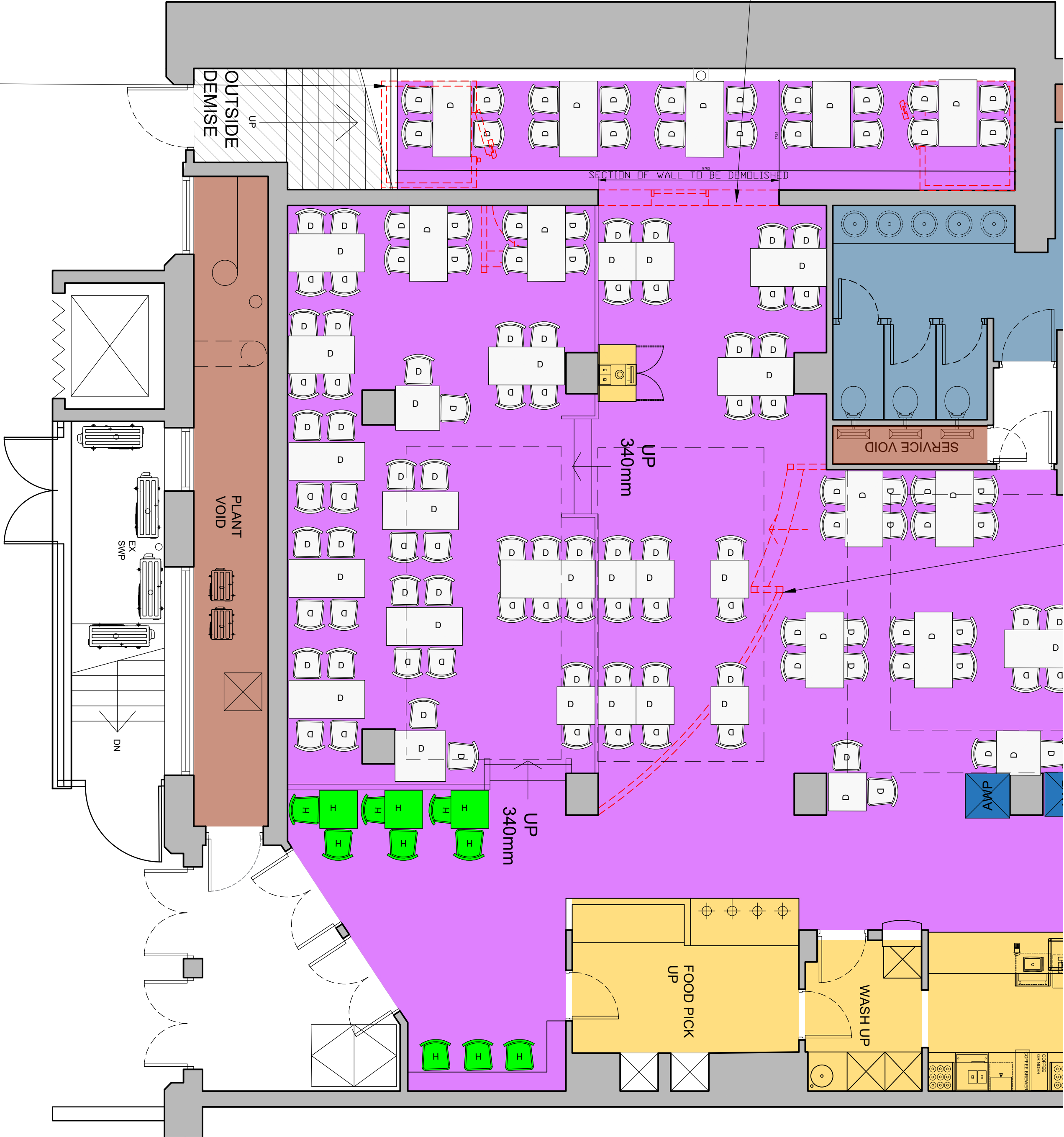
GROUND FLOOR - RAISED CUSTOMER AREA SCALE 1:50
