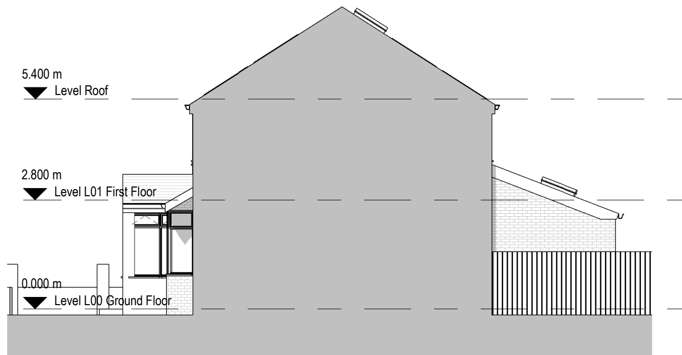
3 Existing South Elevation 1 : 100
