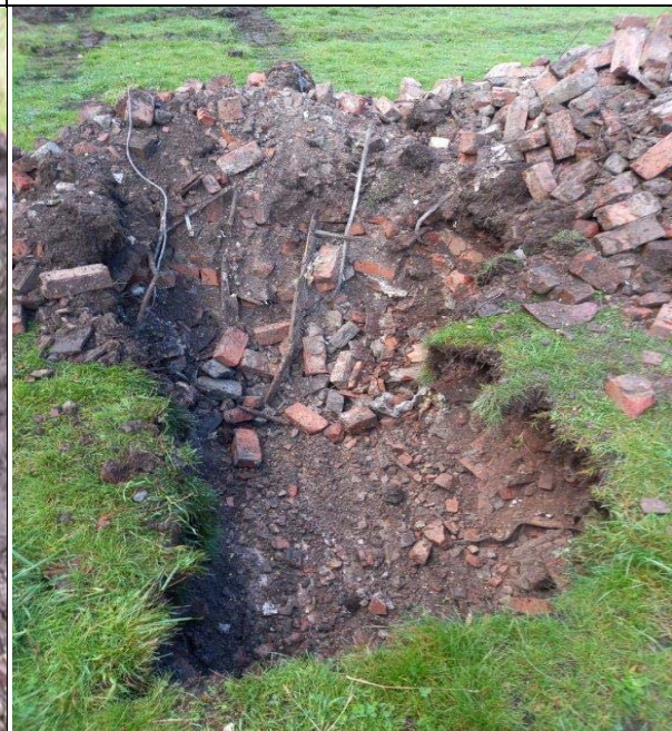
Photo 4: Showing made ground in TP05, facing north.
