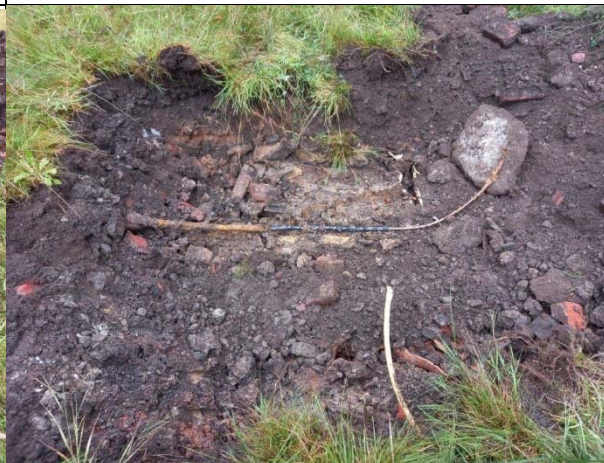
Photo 4: Showing made ground in TP05, facing north.
