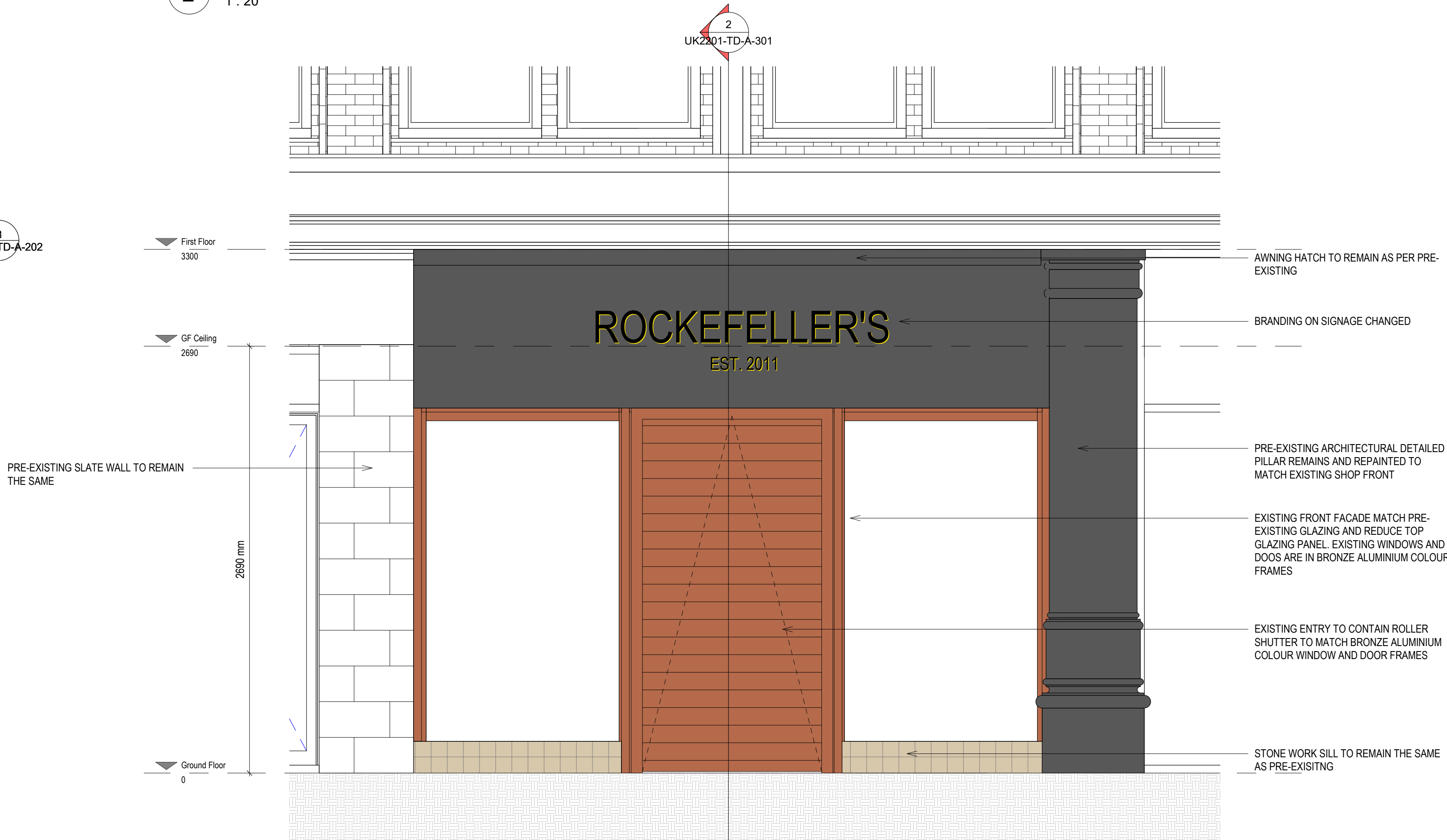
3. EXISTING SHOPFRONT ELEVATION A - CLOSED ROLLER DOOR 1 : 20
