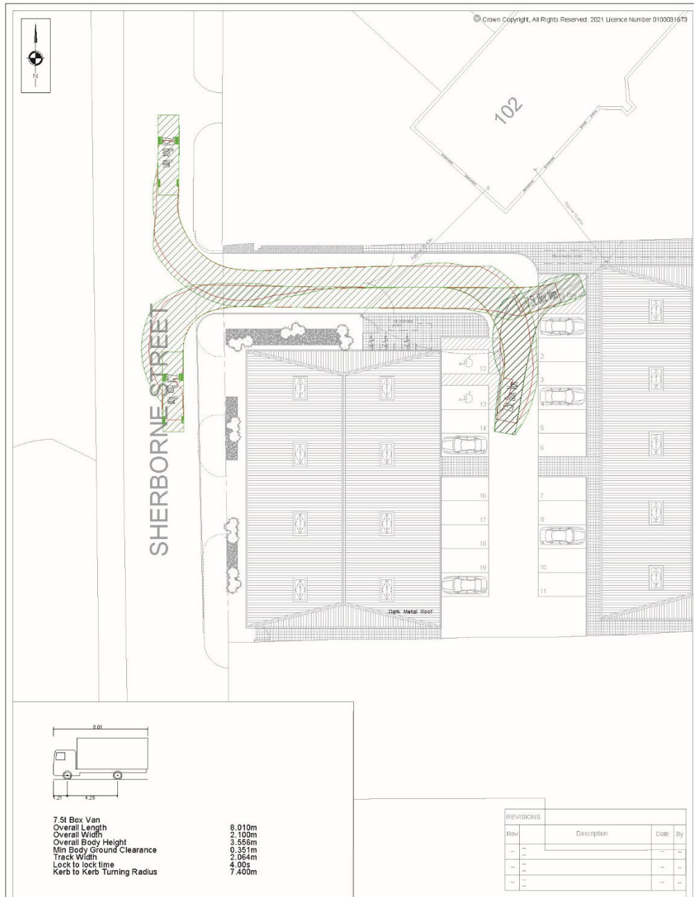
Image 9: Swept path analysis prepared by SCP
