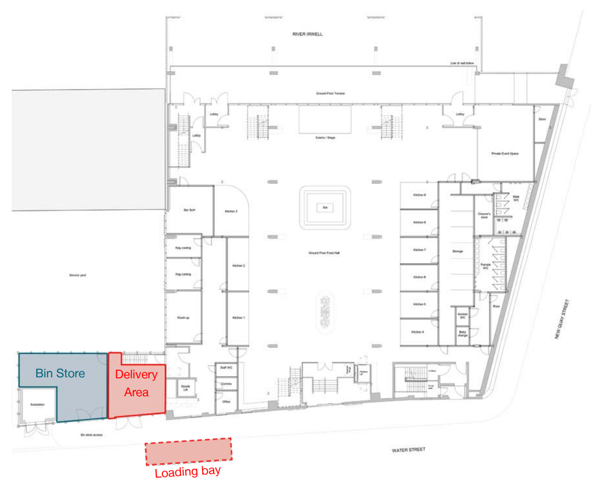
Proposed Building Servicing - (01 First Floor)
