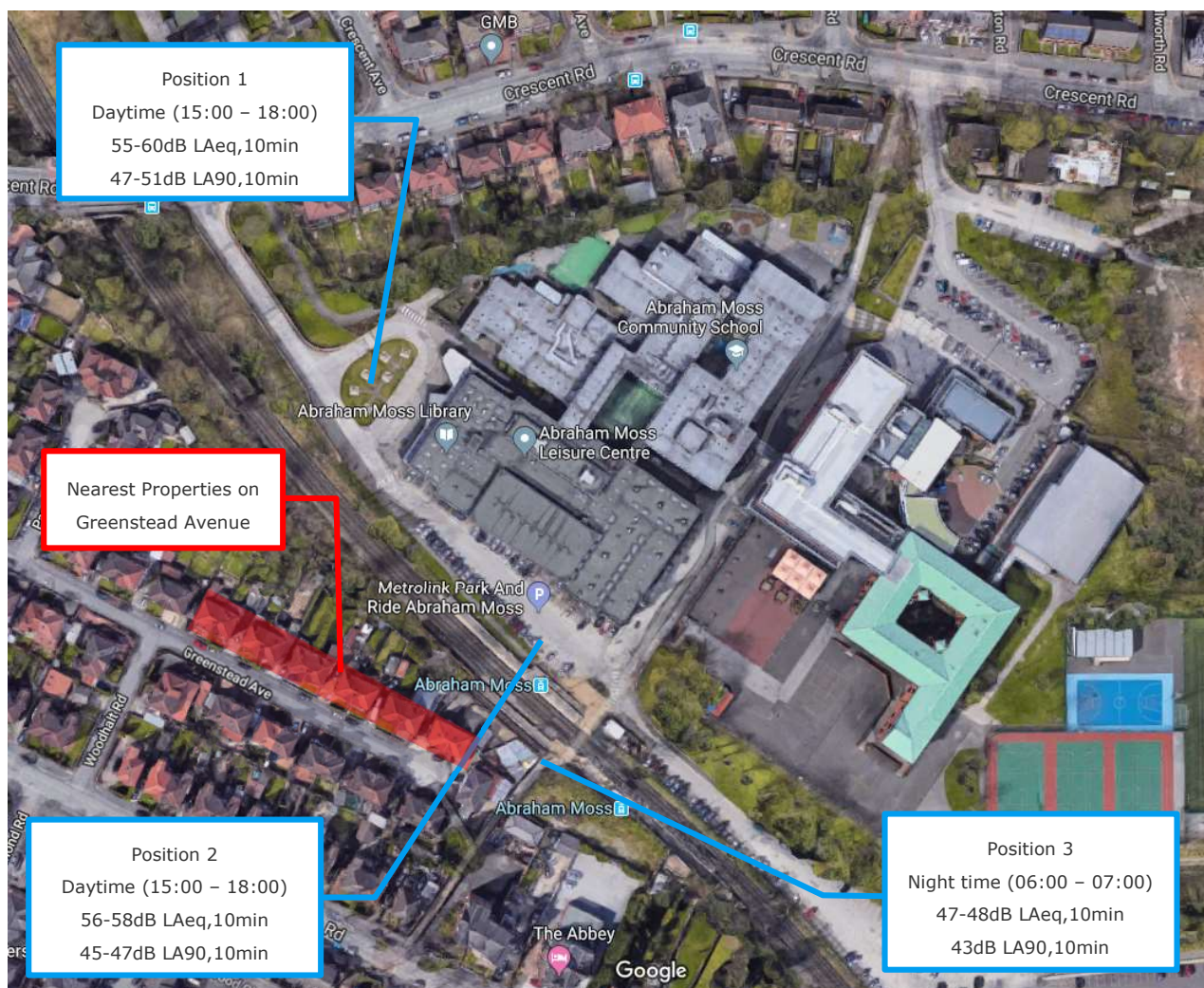
Figure 1 – Noise Measurement Positions and Results
