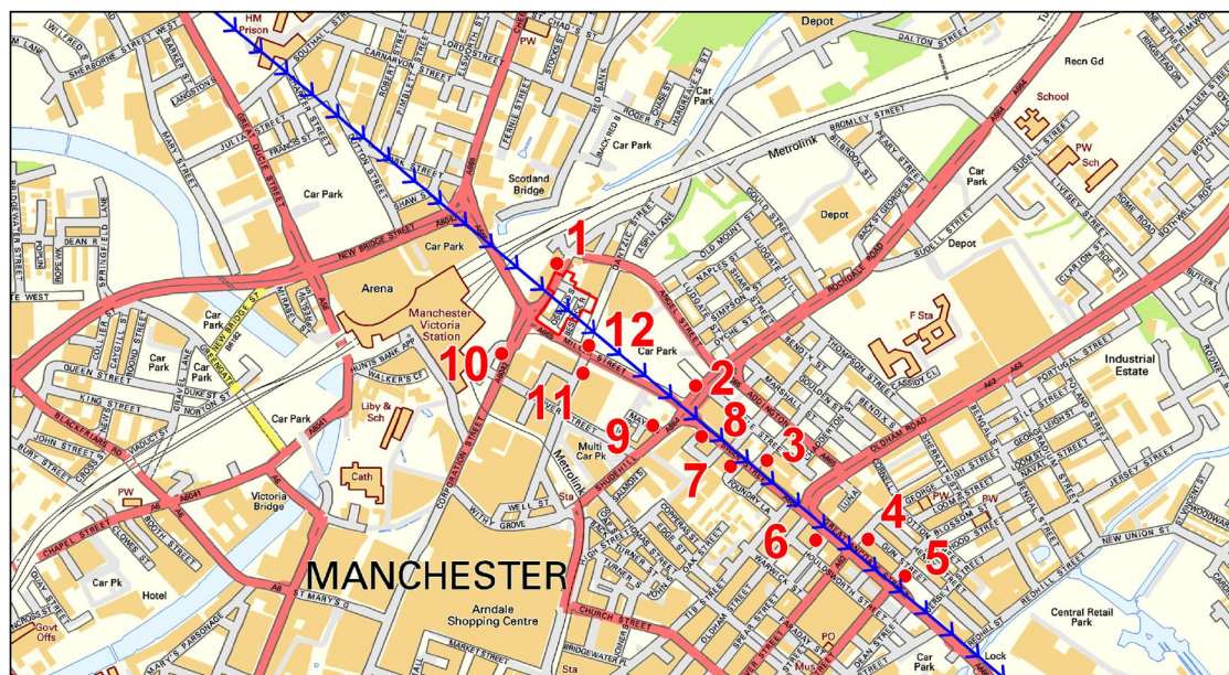
Figure 2 - Surveyed Locations. The blue arrows indicate the direction of the incoming DTT signals from Winter Hill transmitter
