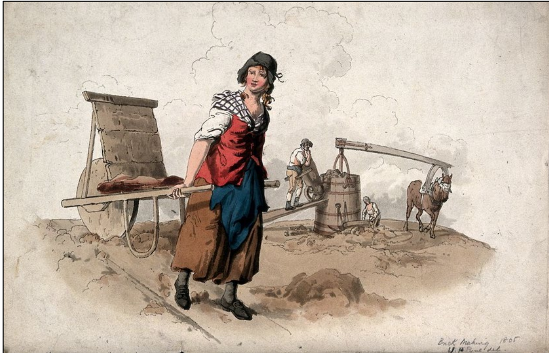
Plate 15: Brickmaking illustration, by William Pyne, showing a young woman taking clay to a vat and a horse in the background powering a stirring mechanism to mix the clay before it is shaped into bricks
