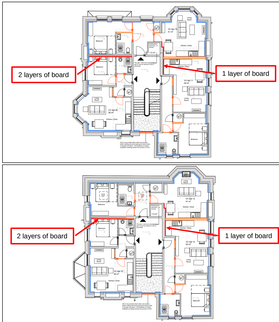
Figure 3.4 - Additional wall linings to first and second floor apartments
