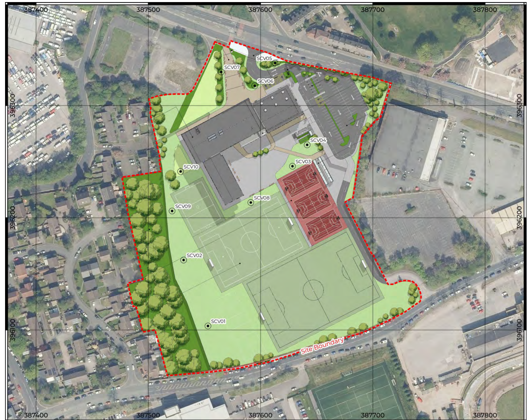
Figure 6 – Soil Cover Validation Pit Layout
