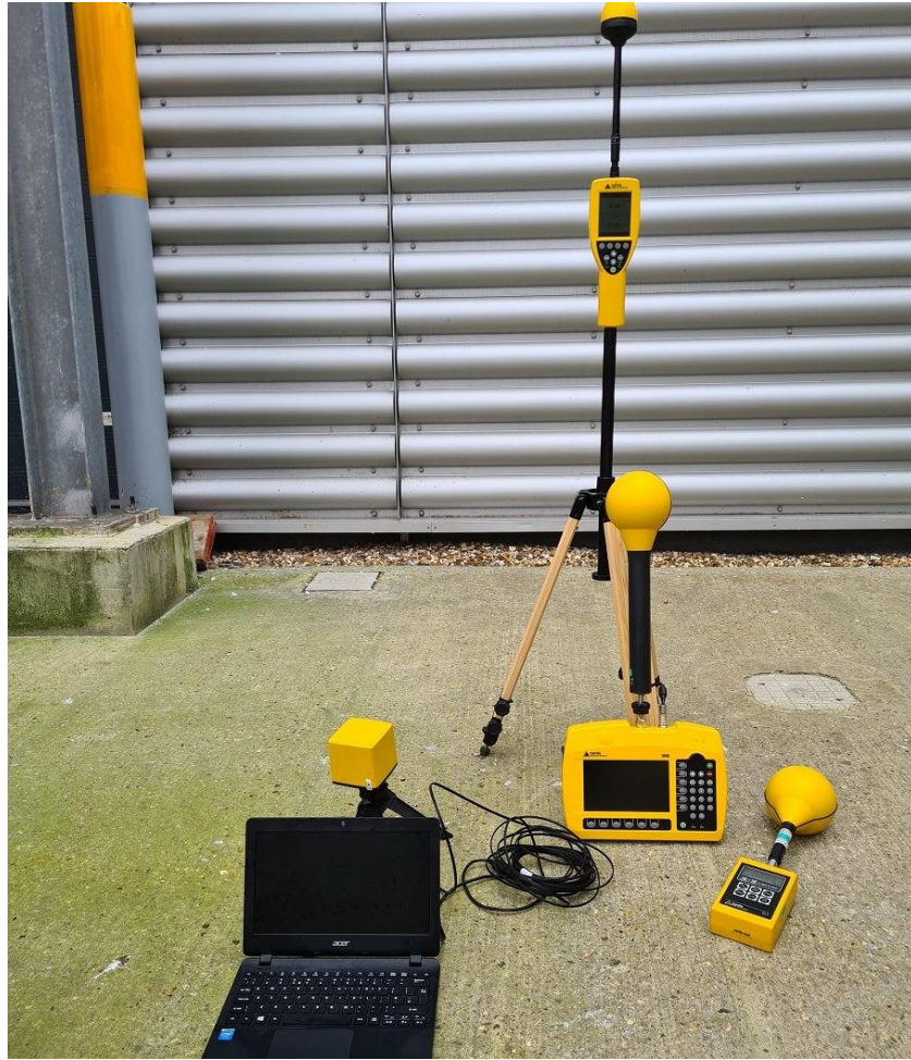
Figure 2.1 Electromagnetic field measurement equipment used during the assessment, including the Narda EHP-50F, Narda ELT-400, Narda NBM-500 and Narda ED-5091.
