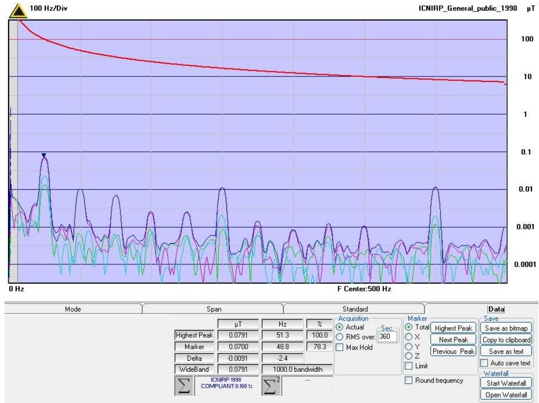
Figure 3.8 Magnetic field spectrum at the boundary between the development site and the substation.
