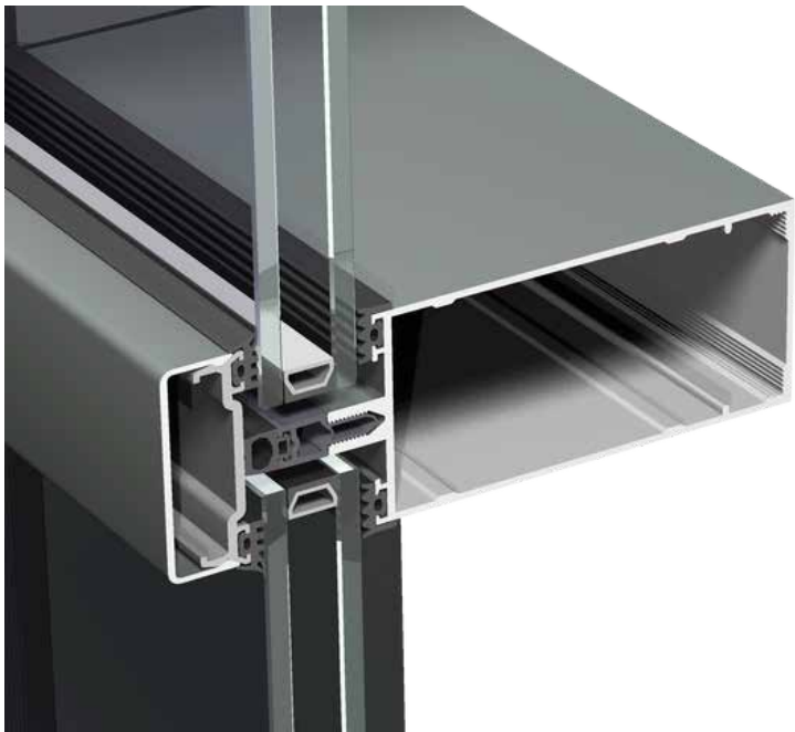
Metal framed glazing system with external capping piece. Note that a single glazed system can be installed within the framework. The Frame can be adapted for opening vents.
