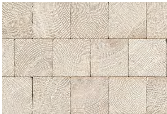
End-grain timber flooring
