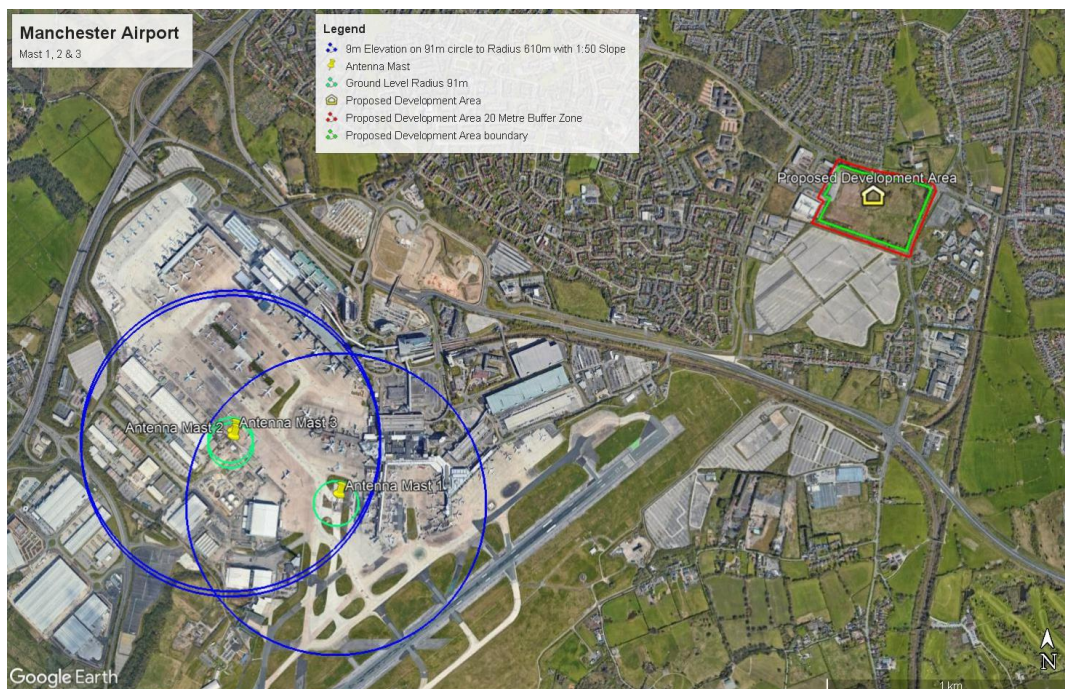
Figure 3 – Antenna Masts 1, 2 & 3 VHF/UHF Communications safeguarding criteria
