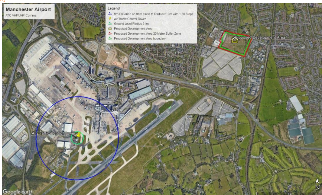
Figure 2 – Air Traffic Control VHF/UHF Communications safeguarding criteria
