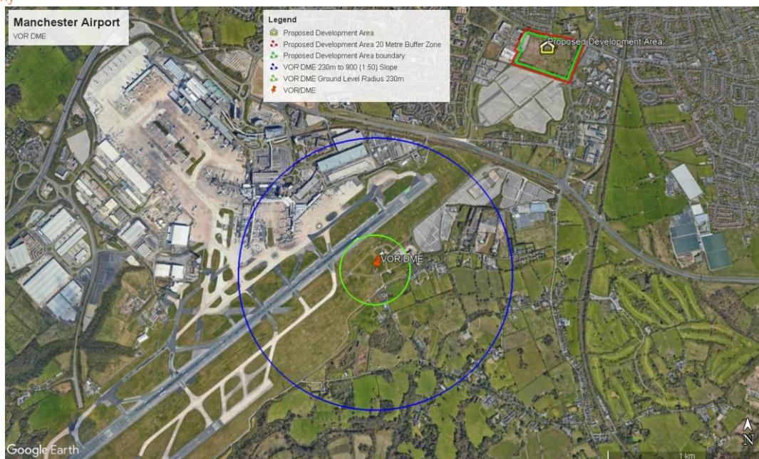
Figure 8 – VOR and DME safeguarding criteria
