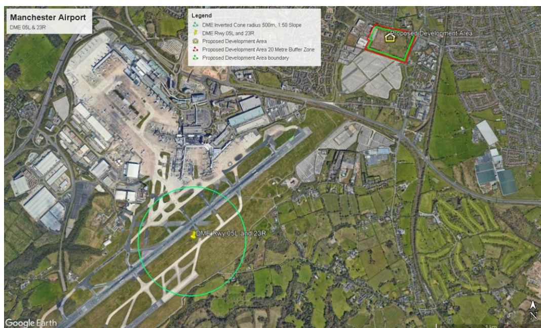
Figure 6 – Runway 05L and 23R DME safeguarding criteria
