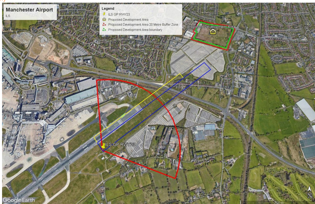
Figure 5 – Runway 23R ILS Glide Path safeguarding criteria
