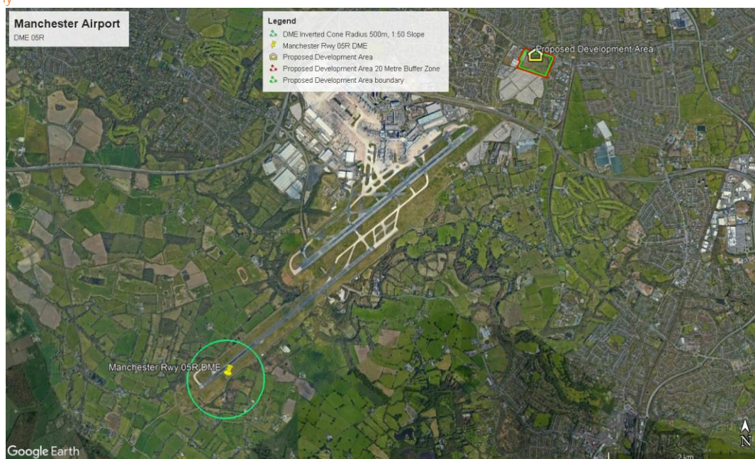
Figure 7 – Runway 05R DME safeguarding criteria
