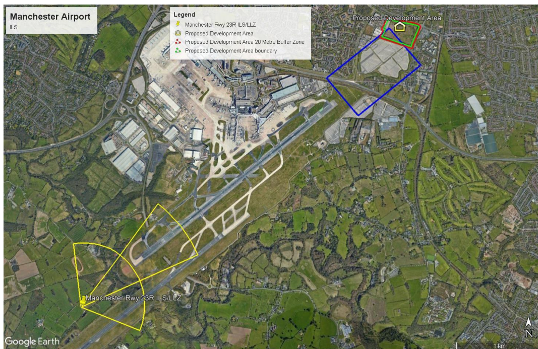
Figure 4 – Runway 23R ILS Localiser safeguarding criteria
