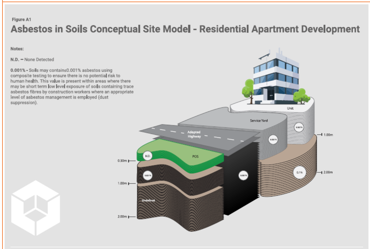
FIGURE 4.1 ASBESTOS RISK MITIGATION CONCEPTUAL SITE MODEL
