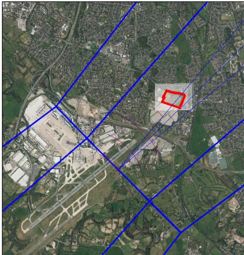
Figure 29 – VOR/DME RWY 23R Protection Area
