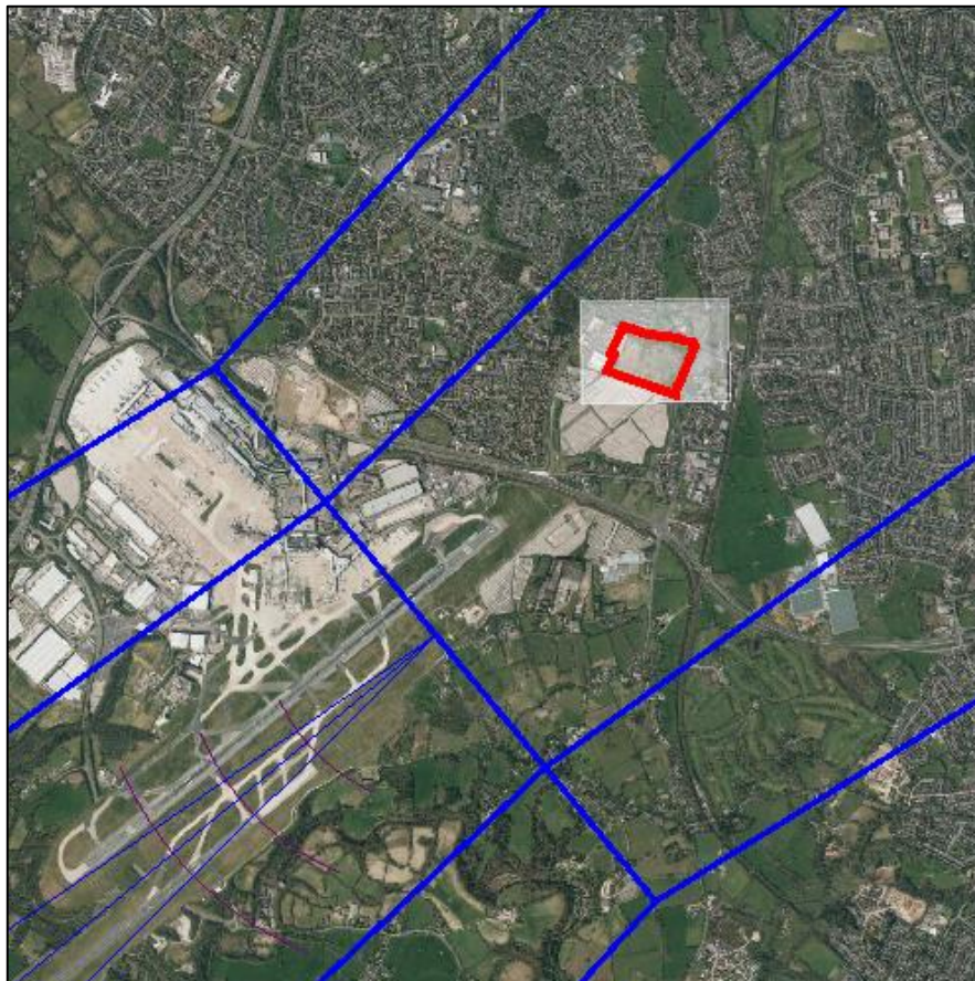
Figure 31 – VOR/DME RWY 23L Protection Area
