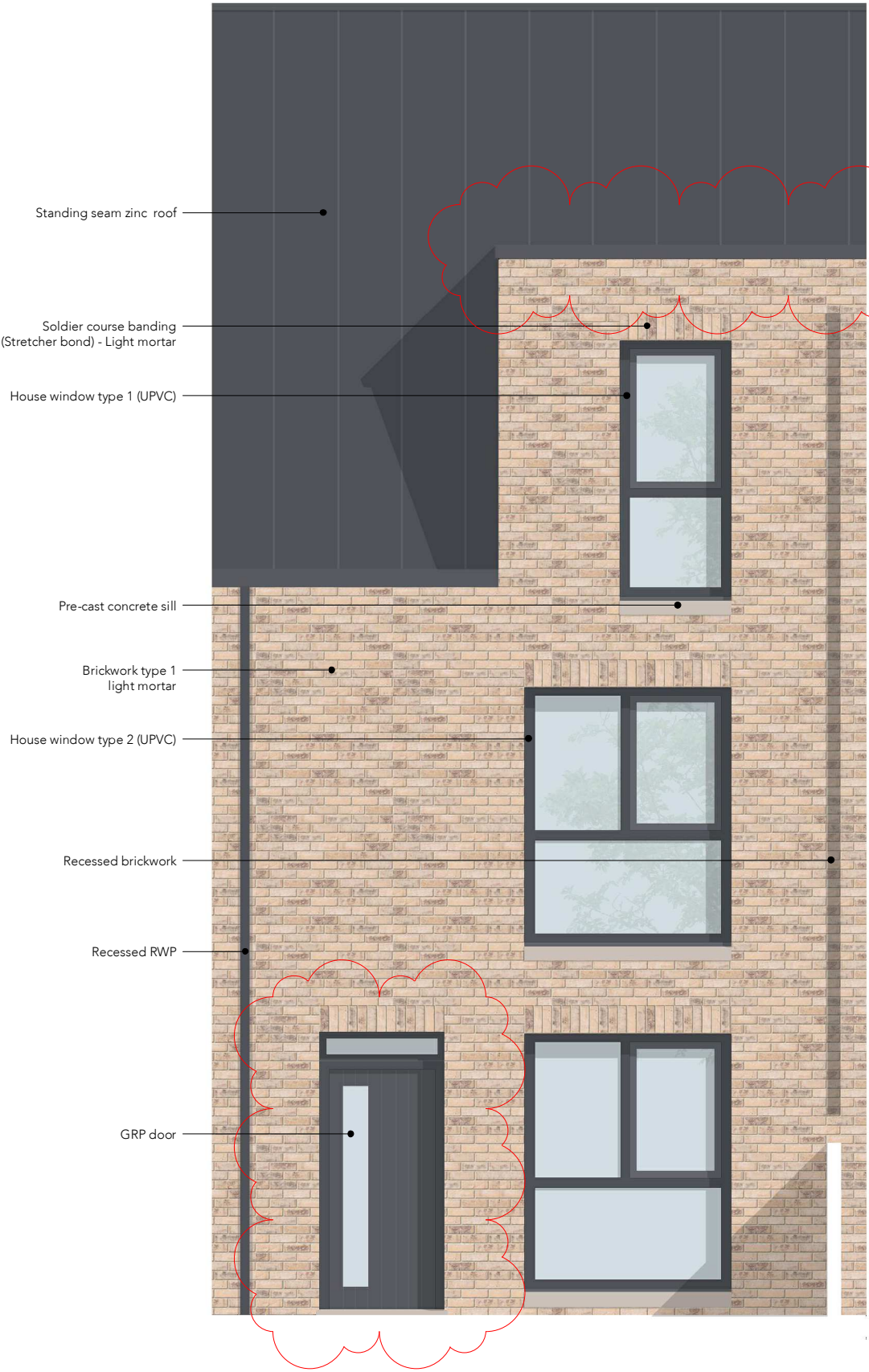
Bay 3 - Houses Full height with opaque panels 1:50
