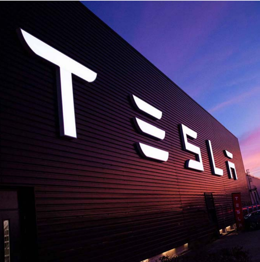
FACE-LIT SIGN WITH PERFORATED VINYL (EXAMPLE)
