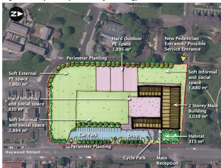
Figure 2.2: Option 1 (Two Storey Building)
