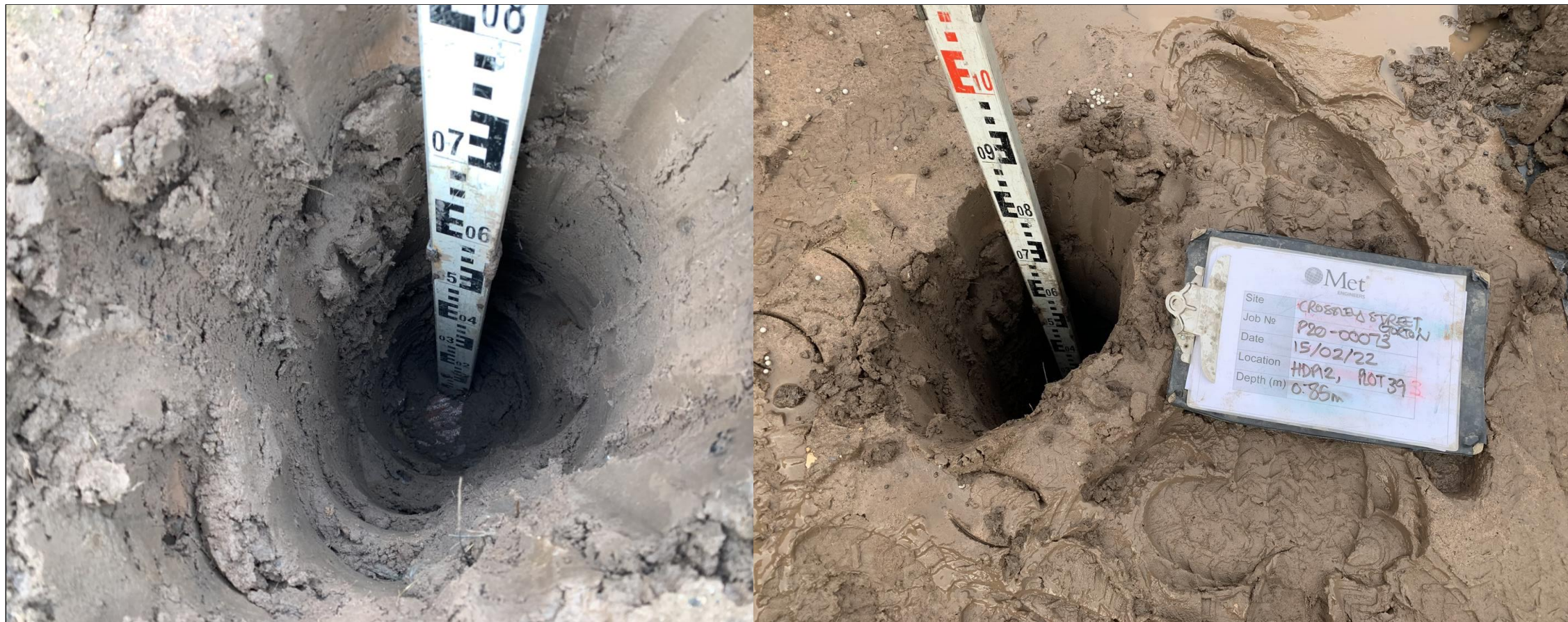
Photographs 9 and 10: Hand Dug Pit Topsoil Depth Validation and Arisings – HDP12, Plot 39
