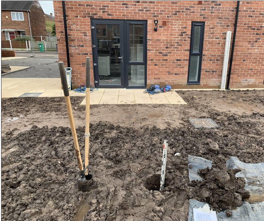
Photograph 7: Hand Dug Pit Topsoil Depth Validation – HDP11, Plot 15
