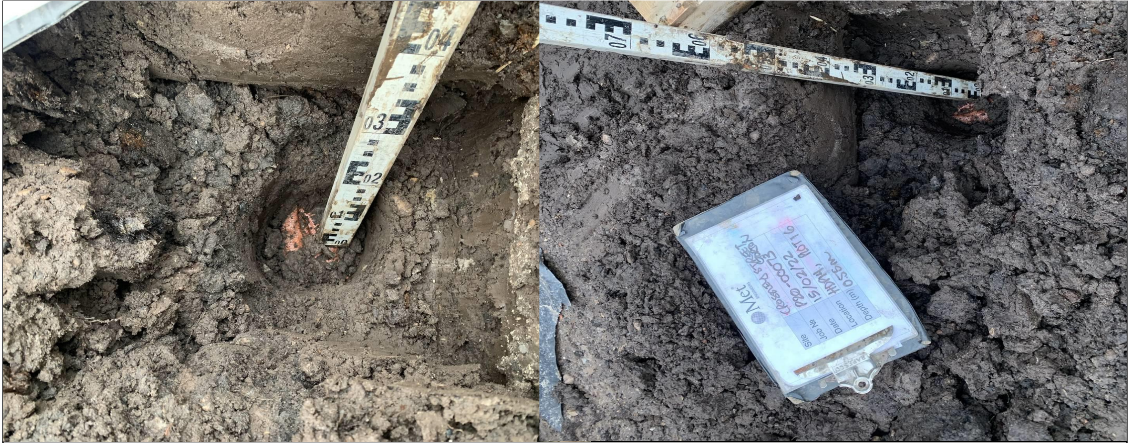
Photographs 17 and 18: Hand Dug Pit Topsoil Depth Validation – HDP14, Plot 16
