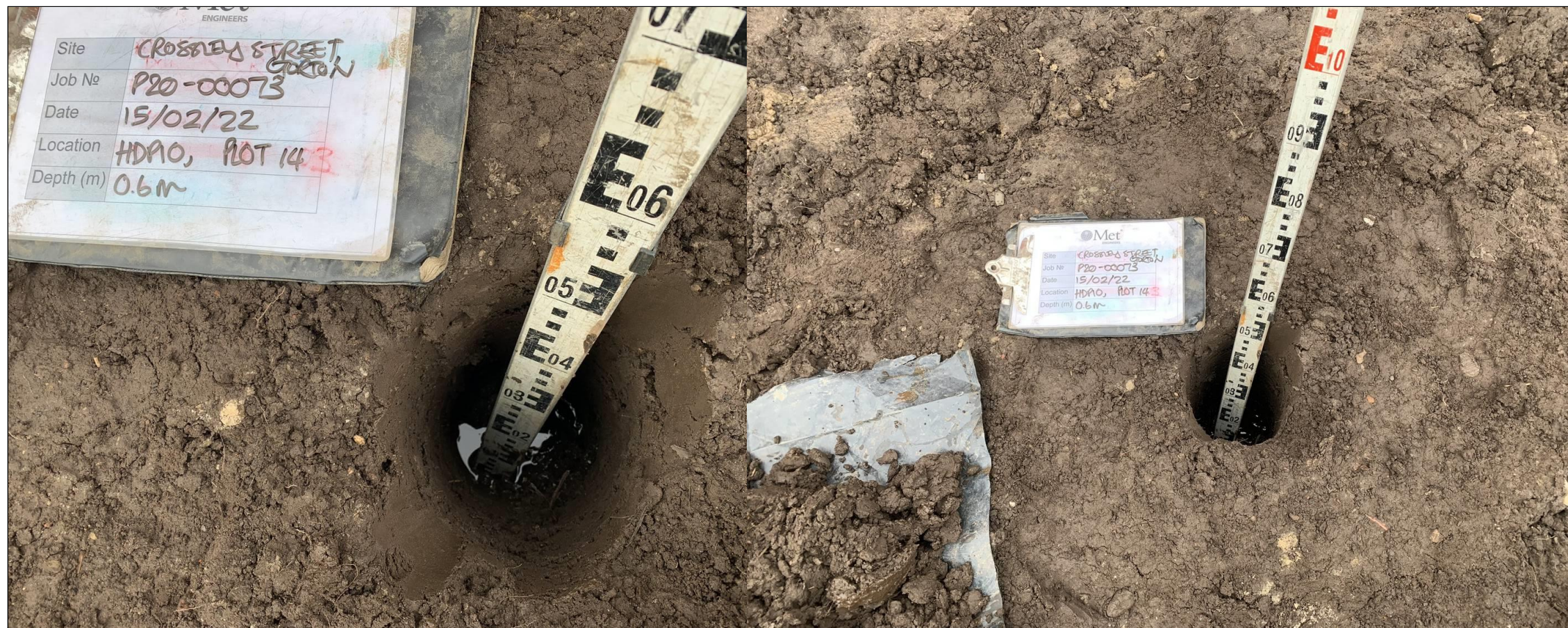
Photographs 1 and 2: Hand Dug Pit Topsoil Depth Validation – HDP10, Plot 14
