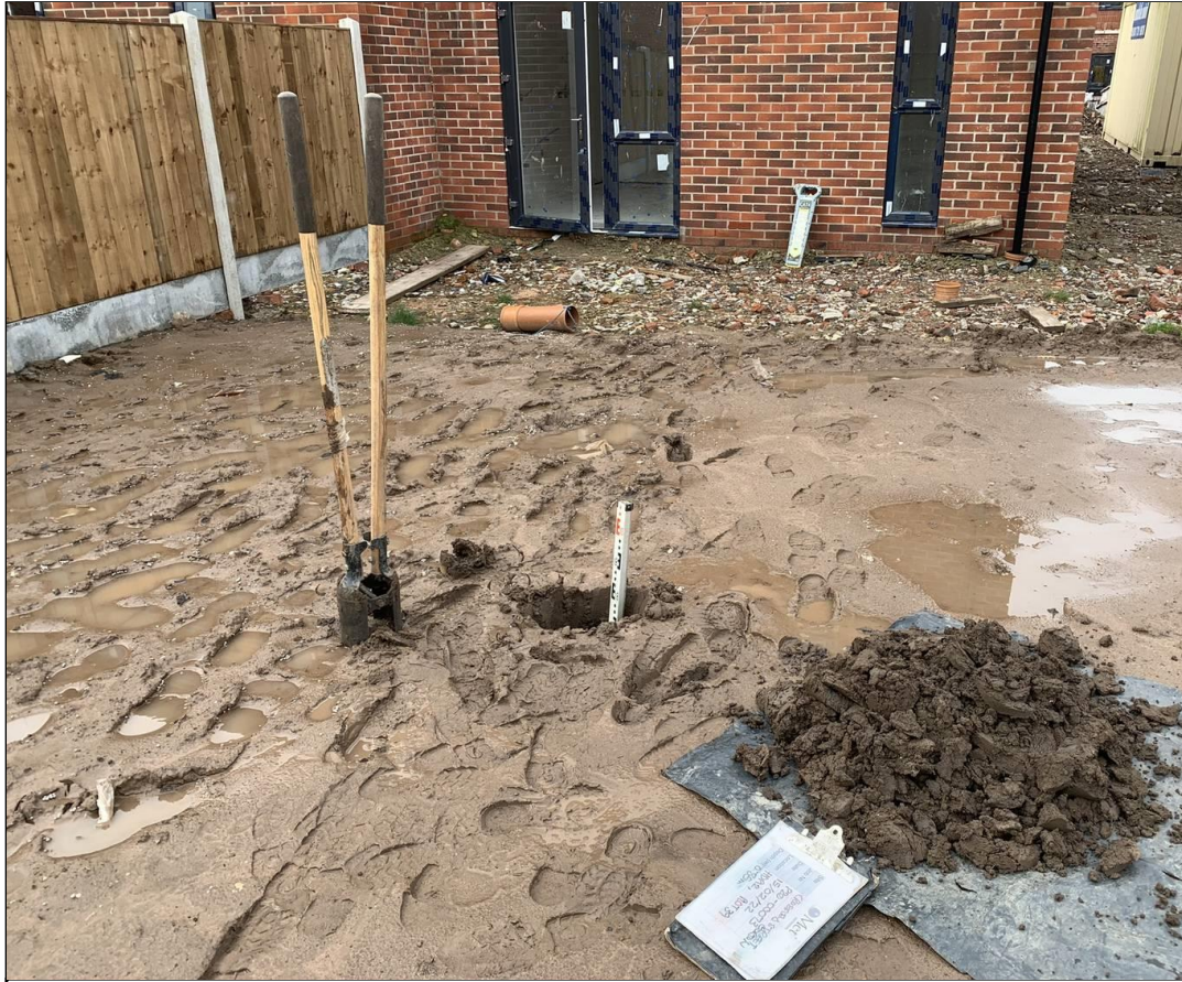
Photograph 11: Hand Dug Pit Topsoil Depth Validation – HDP12, Plot 39
