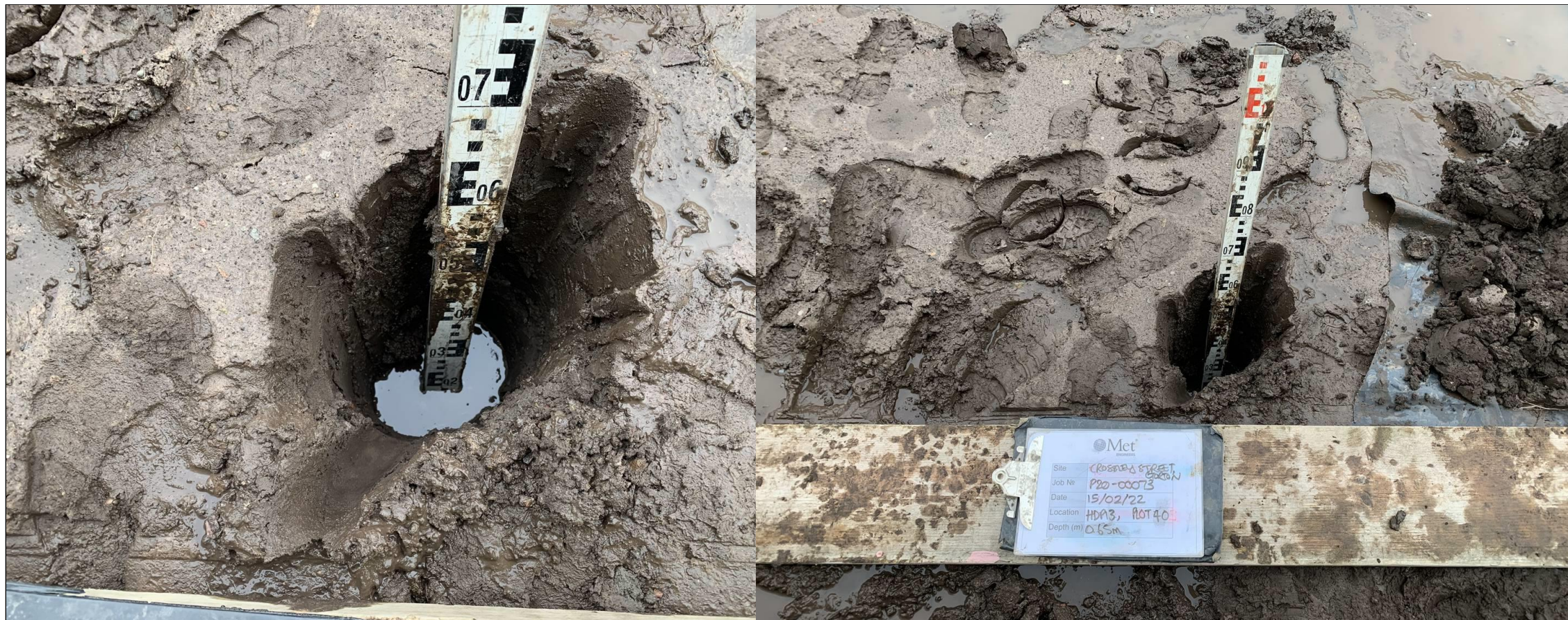
Photographs 13 and 14: Hand Dug Pit Topsoil Depth Validation – HDP13, Plot 40
