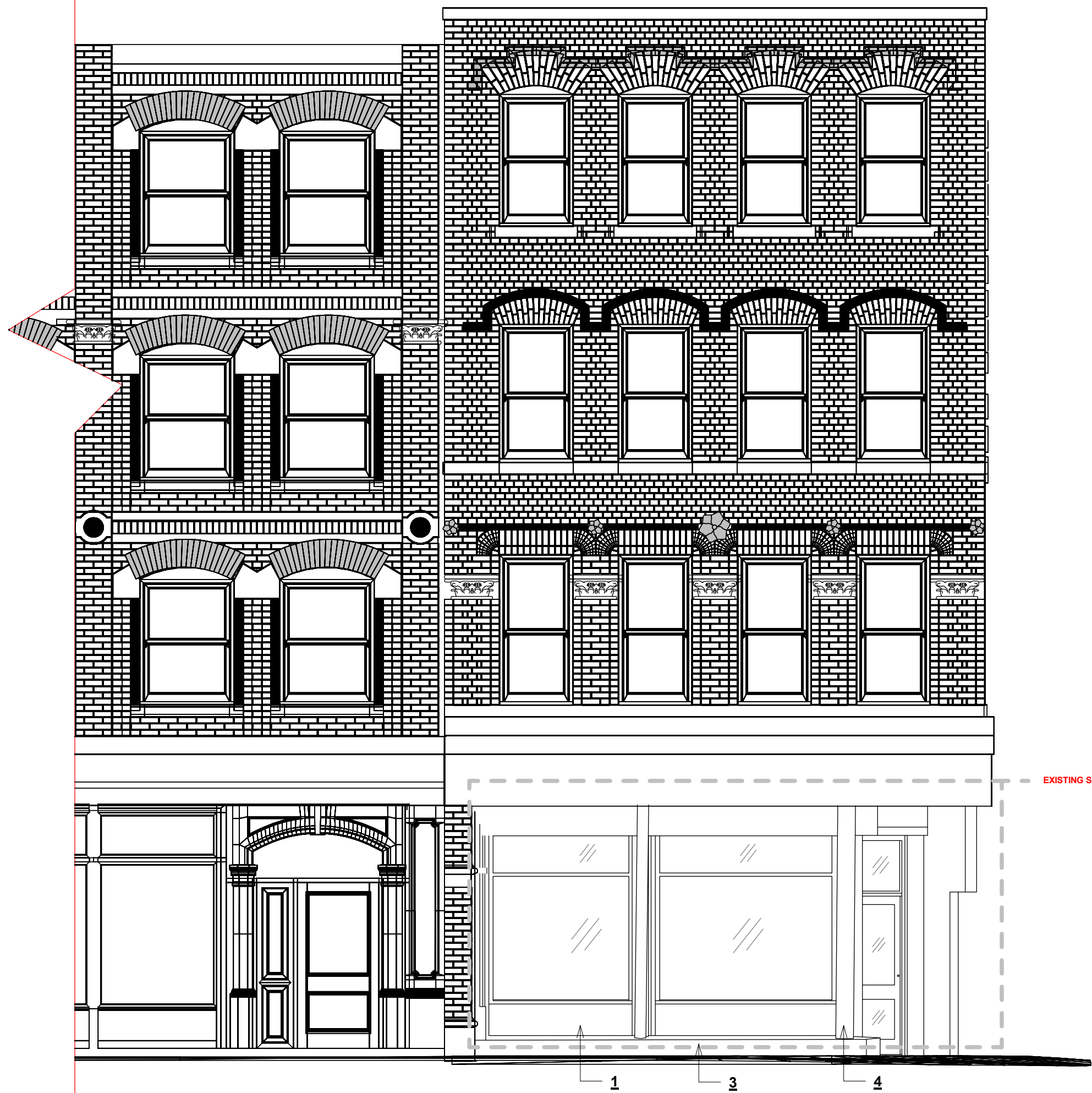
FRONT ELEVATION EXISTING 1:50
