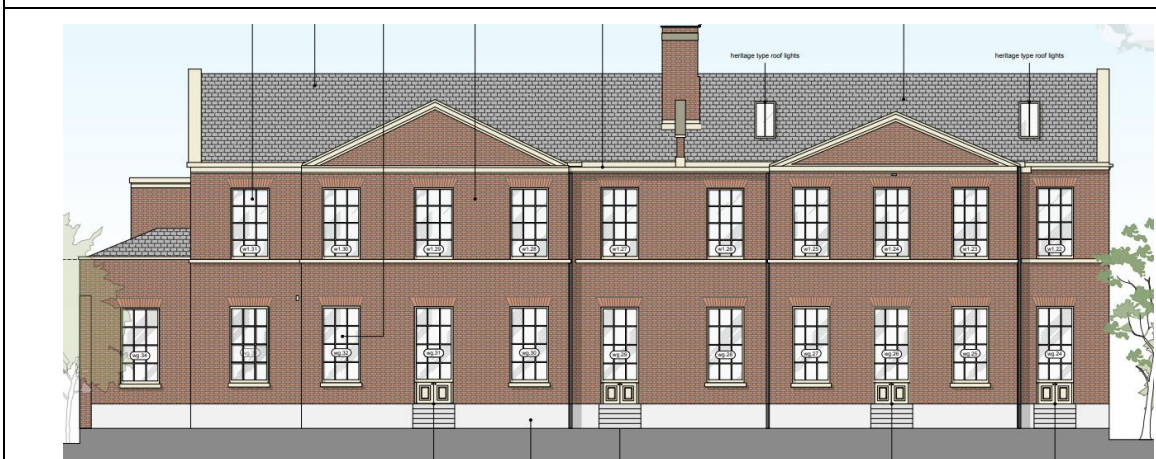
Figure 9 – A cut-away drawing of the proposed east elevation, showing the location and appearance of the four sash window doors, only when viewed from within the narrow private front garden spaces.
