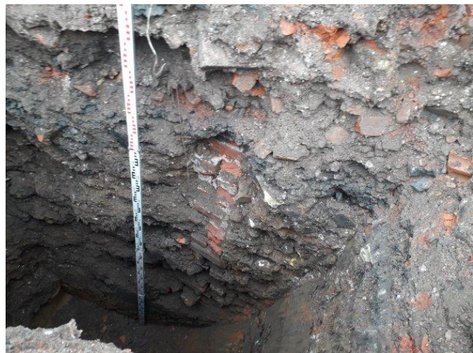
Brick wall visible on south eastern wall of TP204.
