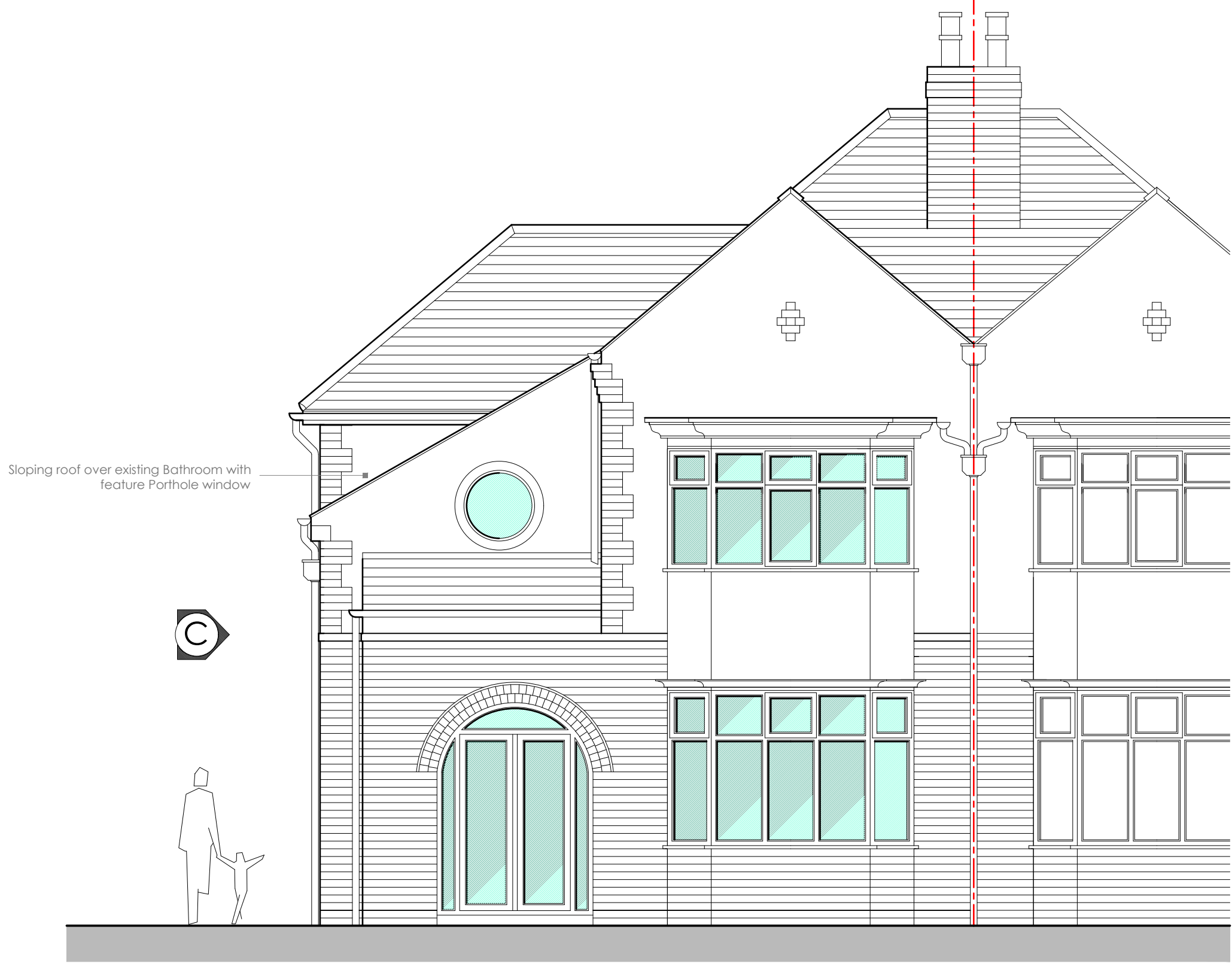
EXISTING FRONT ELEVATION D
