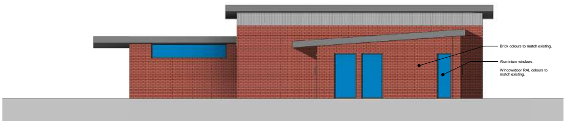
2 Proposed East Elevation 1:50 Ref Sheet: 0200
