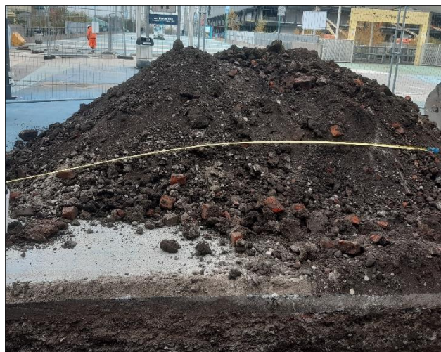
Figure 4-3 Dark brown material located beneath Type 1-style material contains abundant brick and concrete with rare metal and occasional slag.
