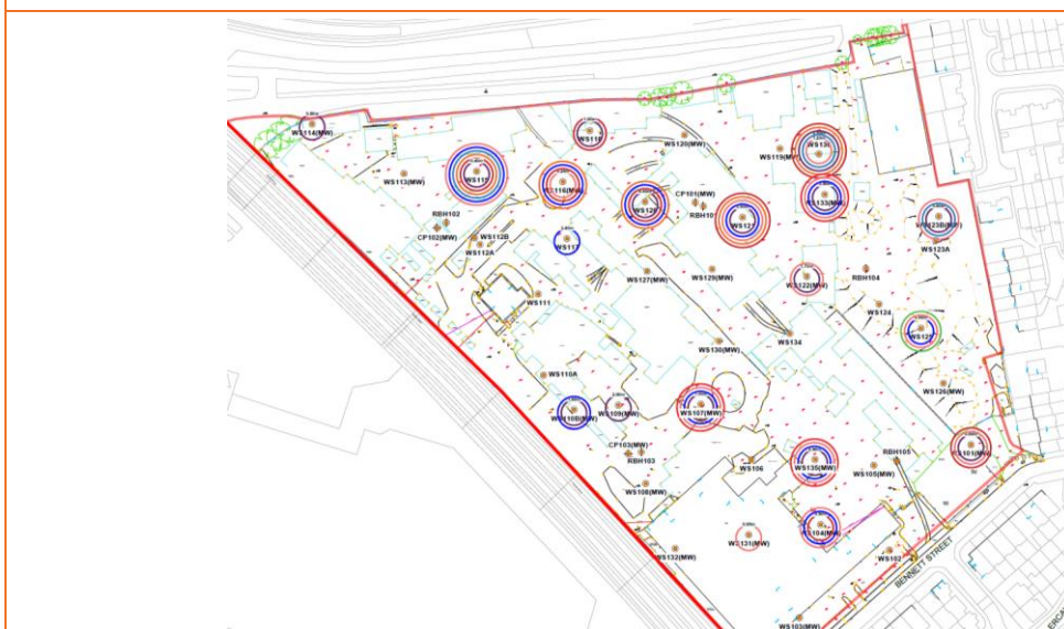
FIGURE 3.3 LOCATION OF IDENTIFIED HYDROCARBON IMPACT
