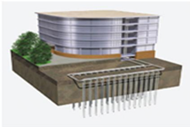
Figure 7: Ground Source Heating
